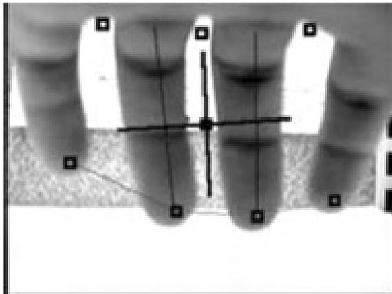
Fig. 2.11 Ahmad and Musilek [1] place a camera underneath the wrist, looking out toward the hand, to interpret finger and arm gestures. © IEEE 2006.
