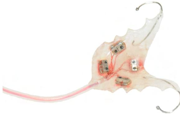
Fig. 2.13 Saponas et al. [125] use retainer-mounted infrared sensor and emitter pairs to classify tongue gestures. © ACM 2009.
