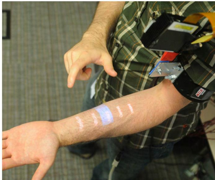
Fig. 2.23 Harrison et al.'s *Skinput* system combines piezoelectric accelerometers (worn in an armband) with a shoulder-mounted projector to prototype an on-body UI [45]. © ACM 2010.
