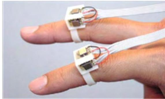
Fig. 2.4 Lam et al. [72] placed accelerometers on rings, wired to a radio transmitter (not shown) worn on the wrist. © IEEE 2003.
