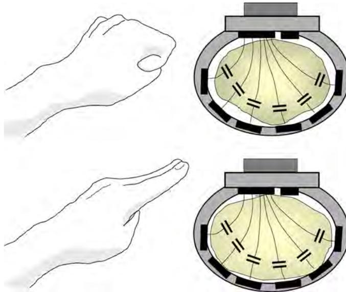
Fig. 2.26 Rekimoto's *GestureWrist* system [111] leverages the fact that the wrist changes shape — and therefore changes its electrical properties — when hand posture changes. © IEEE 2001.
