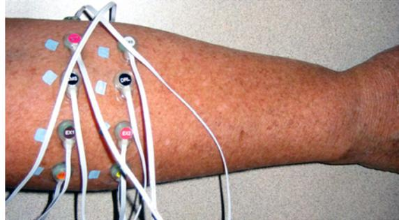
Fig. 2.20 Surface electromyography (sEMG) allows non-invasive measurement of electrical muscle activity [117]. © ACM 2008.
