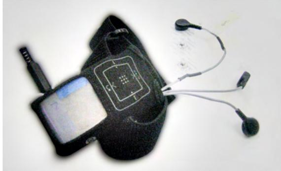
Fig. 2.22 Costanza et al. [25] integrate EMG electrodes into an armband form factor that might be plausible for consumer use. © ACM 2007.
