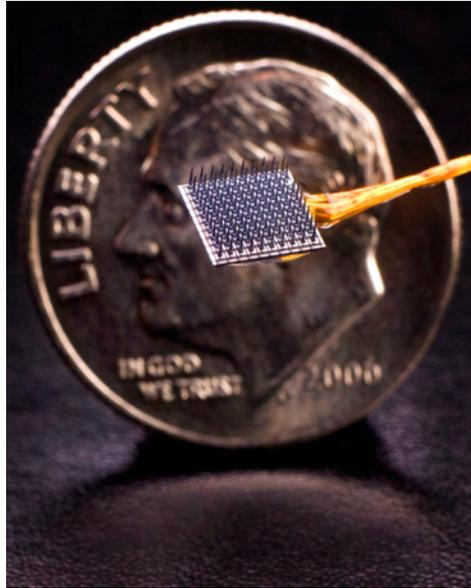
Fig. 2.14 Intracortical electrode arrays are surgically placed on the surface of the brain, and can record the electrical activity of several hundred brain cells. Image courtesy John Donoghue and Matthew McKee/BrainGate Collaboration.
