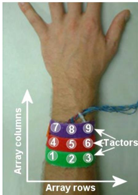
Fig. 3.1 Oakley et al. [94] use a  $3 \times 3$  array of haptic actuators to explore perceptual questions around a plausible form factor for wearable haptics. © IEEE 2006.
