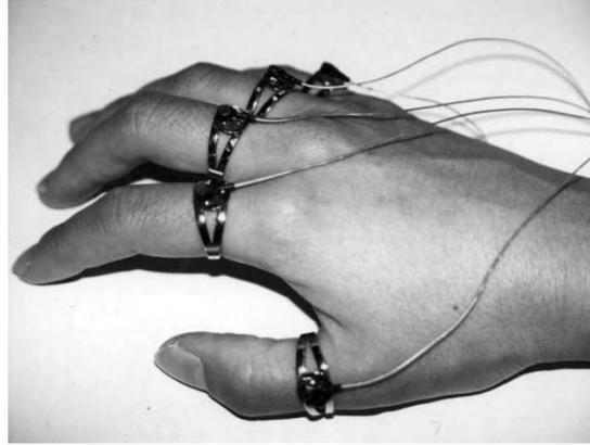
Fig. 2.3 Fukumoto and Suenaga [32] placed accelerometers on the fingers to detect gestures and contact with surfaces. © ACM 1994.
