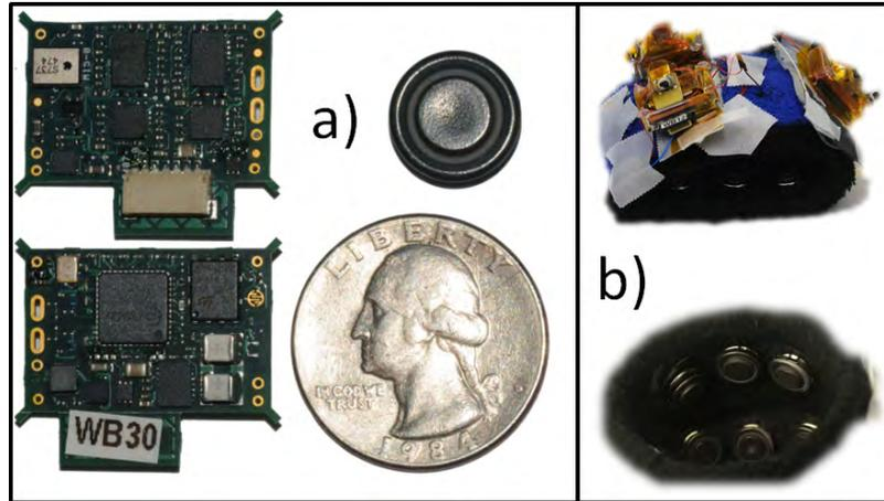
Fig. 2.21 Saponas et al. present a wireless, dry sEMG device [116]. © ACM 2010.
