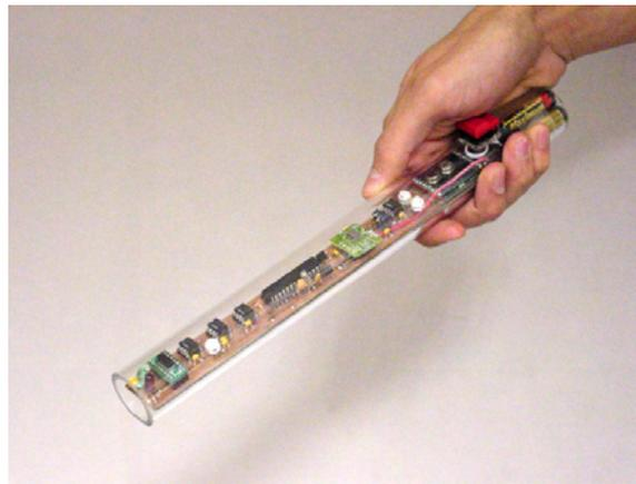
Fig. 2.1 Wilson's and Shafer's XWand [148] combined accelerometers with a gyroscope and a magnetometer. Image © ACM 2003.
