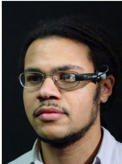
Fig. 3.2 The Teleglass project provides an LCD display that clips on to any pair of eyeglasses. Courtesy Hrvoje Benko and Alex Olwal.
