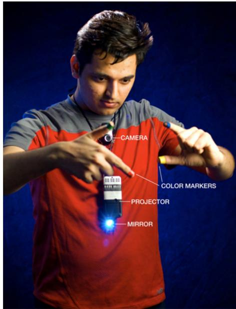
Fig. 2.9 The SixthSense project [86] envisions a color camera worn on a pendant that uses computer vision to recognize hand gestures. Courtesy Pranav Mistry.
