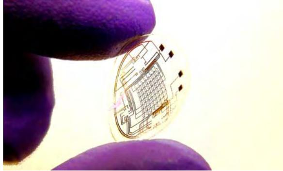
Fig. 3.4 Saeedi et al. are working toward embedding displays directly on contact lenses. Courtesy Babak Parviz.
