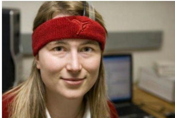
Fig. 2.17 Functional near-infrared spectroscopy is non-invasive and inexpensive, but probably lacks the bandwidth for direct-control brain–computer interfaces. © ACM 2009.
