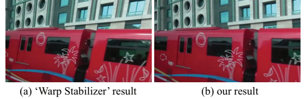
(a) 'Warp Stabilizer' result (b) our result Figure 15. Comparison with Adobe After Effects CS6 'Warp Stabilizer'. We can notice the global shearing/skewing in 'Warp Stabilizer' results.
