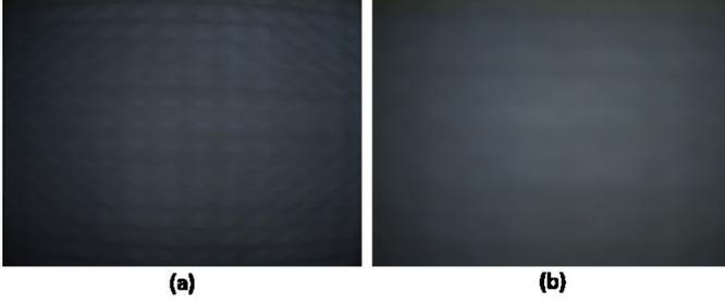
**Fig. 6.** Images of a pure white paper in front of the lens. (a) 6mm lens. (b) 12mm lens.
