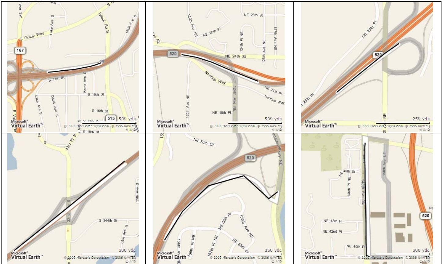
Figure 9: Parallel road distraction. Parallel roads or lanes of opposing traffic often distract the nearest road algorithm, while ours stays on a more likely path.
