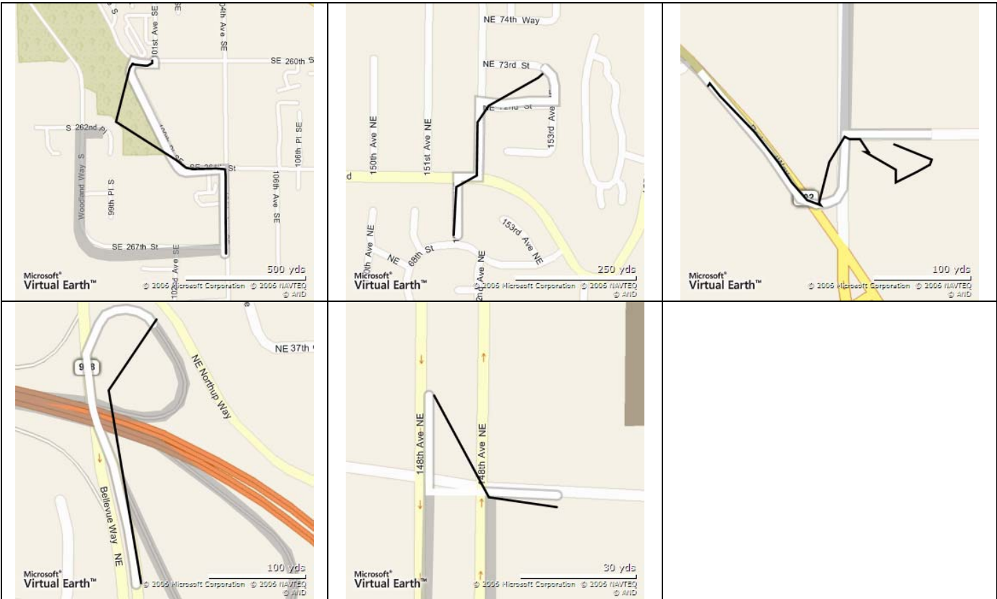
Figure 8: GPS problems. Our technique gives good results in spite of inaccurate and under-sampled GPS.
