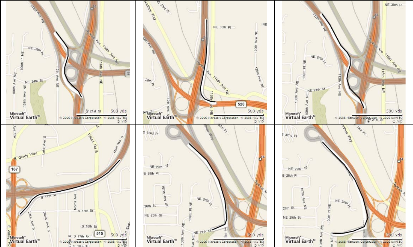
Figure 12: Spaghetti bypass. Our algorithm avoids being drawn into complex interchanges when the actual route passes by.
