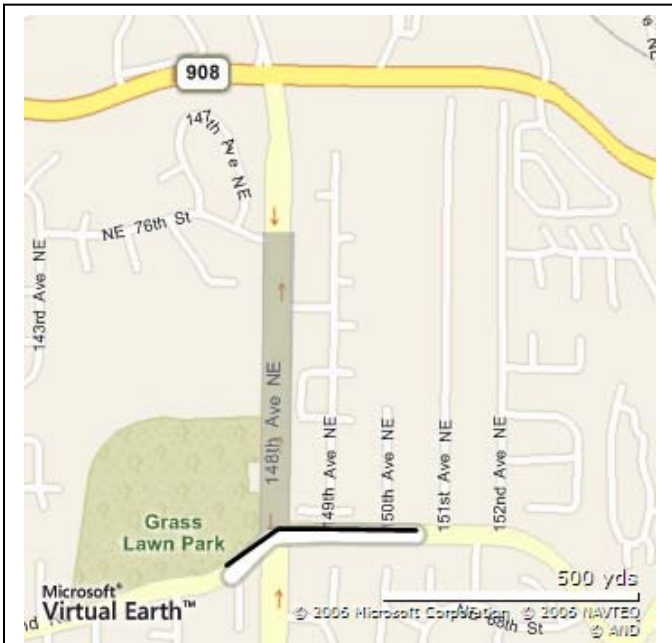
Figure 2: Nearest road matching fails in this example. The black line connects the measured GPS points. When the path crosses the north/south street, nearest road matching matches it, ignoring the path's continuity and implying an eventual U-turn, shown in gray. Our algorithm gives the white route.
