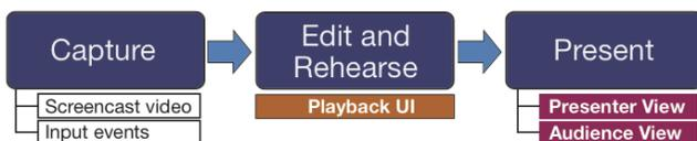
**Figure 2. DemoWiz workflow:** Presenters captures a software demonstration, edit the recording while rehearsing with our playback UI, and present the edited video to the audience using a presenter view.
