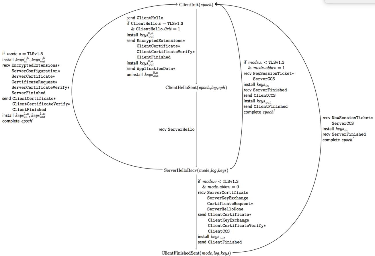
Fig. 5: Composite client state machine for TLS 1.0-1.3, covering full and abbreviated handshakes, client authentication, and 0-RTT early data. Messages labeled with \* may be skipped depending, for example, on the negotiated handshake *mode*.
