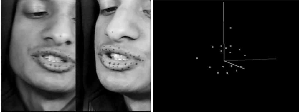
Figure 3-6: An input frame and the reconstructed 3D points
