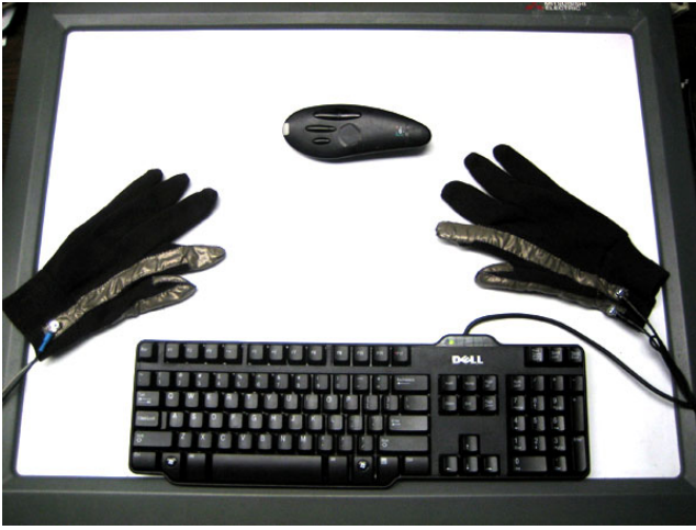
Figure 5: Interaction devices used in our experiment (top to bottom): A 3DOF tracked three button wand (Logitech TrackMan Live), a pair of specially constructed gloves with two active fingers on each hand, and the keyboard. The devices are laid out on the DiamondTouch surface.
