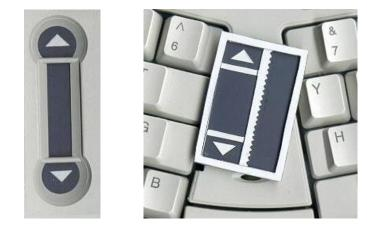
Figure 1: Some alternative physical embodiments of the touch-sensitive strip.
