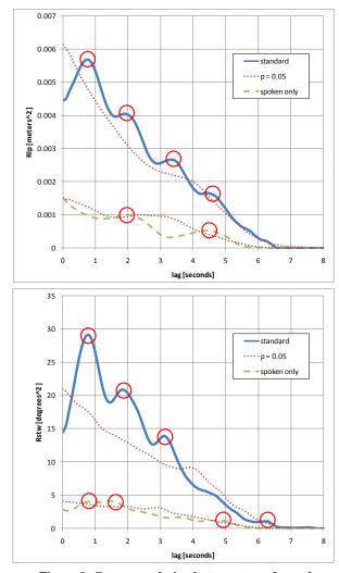
Figure 9. Cross-correlation between transformed instantaneous PDT on the outside world and lane position variance (top) and steering wheel variance (bottom). Calculated only using gazes away from the outside world of 200 ms or longer. Circled peaks indicate statistically significant increases in variance occurring after decreases in the IPDT, with the delay indicated by the value of lag.
