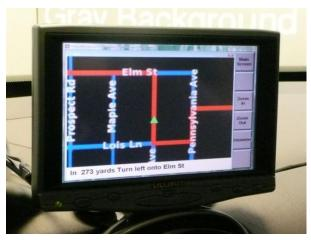
Figure 3. LCD screen displaying real-time location of the vehicle on a map.
