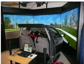
Figure 1. 180° field of view driving simulator.
