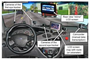
Figure 2. Experimental setup inside the vehicle.
