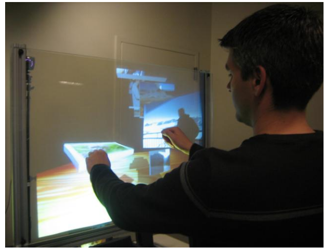
Figure 3. Interacting with DepthTouch : user’s left hand is touching an object of interest, while his right hand is adjusting the orientation and depth of that object by moving in mid-air above the surface.
