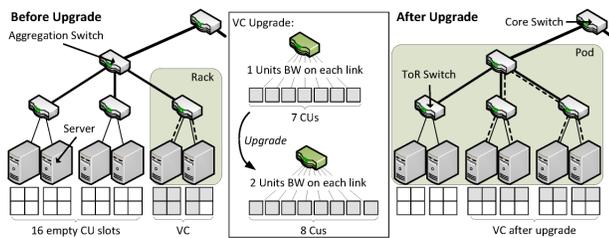
Fig. 2: Upgrade of a virtual cluster VC: *Left* - the initial state: VC(7,1) is embedded on the right-most rack of a pod of the fat-tree. The dashed lines indicate the current bandwidth reservations. *Middle* - the upgrade request: VC(7,1) needs to be upgraded to VC(8,2). *Right* - after the upgrade: Three CUs were migrated in order to find a new feasible embedding of VC which does not violate the capacity on the servers' uplinks.
