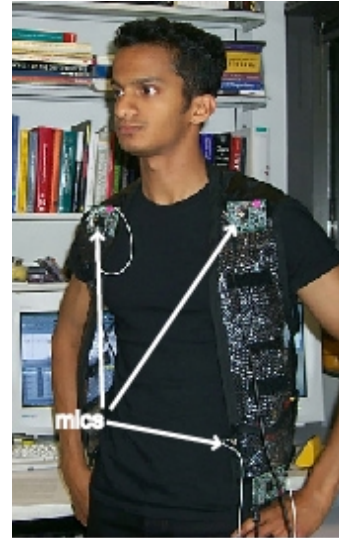
Figure 3. Initial implementation of wearable phased array.
