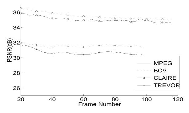
Figure 10: Comparison of coding PSNR between BCV scheme and MPEG-I scheme
