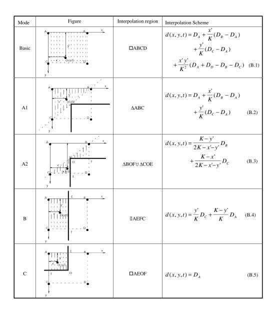
Figure 2: Summary of interpolation rules for BCV motion field representation, where A, B, C and D denote four control points,  $D_A$ ,  $D_B$ ,  $D_C$  and  $D_D$  are the associated control vectors, and a solid line indicates the presence of boundary discontinuity.
