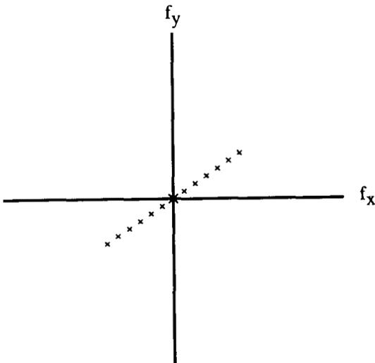
Fig. 9. Fourier transform of grating.
