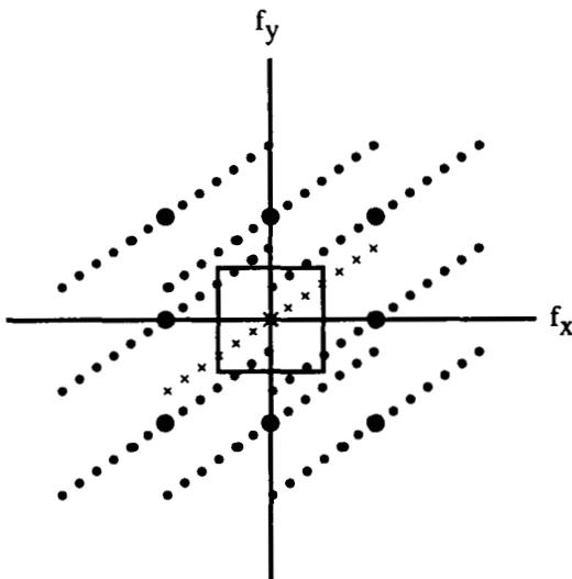
Fig. 10. Spectral orders after first stage sampling.
