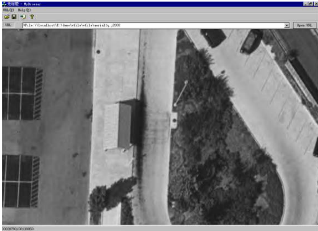
Figure 9 Vmedia interactive image browser as an independent application. The browsed image is Aerial1, the largest image in the standard JPEG 2000 test set. The original image is of size 14565x14680. It is compressed to 1.0bpp or 26,101 KB. The interactive browse window is of size 1020x630
