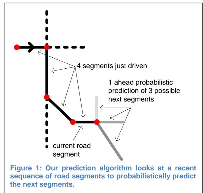
Figure 1: Our prediction algorithm looks at a recent sequence of road segments to probabilistically predict the next segments.
