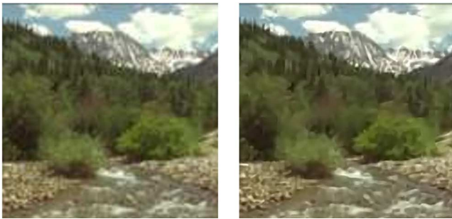
Fig. 16. Super-resolution result of an image with rich texture regions. Left: bicubic interpolation, and right: our approach.
