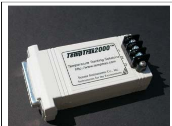
Figure 1: We use this RS-232 thermometer to measure ambient temperature.
