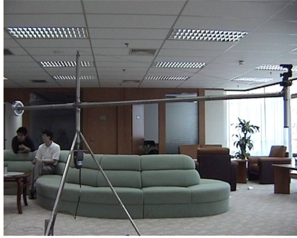
Figure 1: Capturing device of concentric mosaics.
