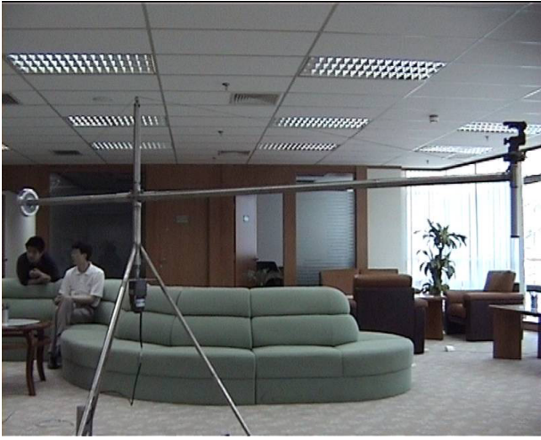
Figure 1: Capturing device of the concentric mosaic.
