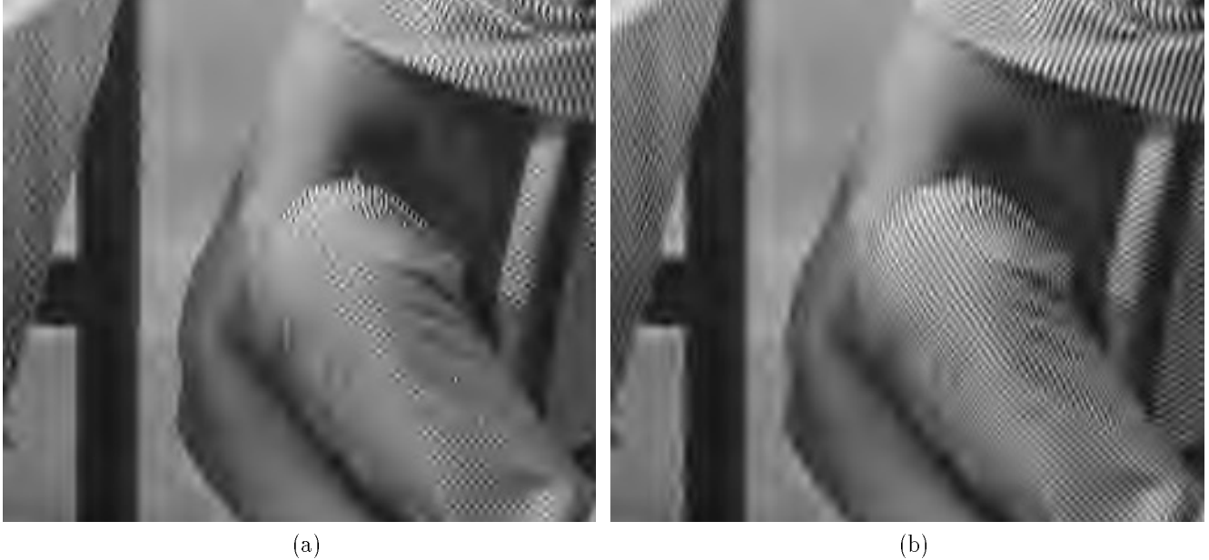
Figure 4: Experimental results for Barbara of (a) the coded image with LZC, and (b) the coded image with R-D optimized wavelet packet transform.
