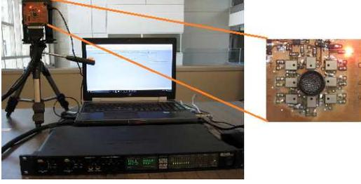
**Fig. 1:** Left: Hardware Set-Up; Right: Ultrasonic piezoelectric transducer at the center and an 8-element microphone array around it in a circular configuration.
