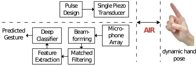
**Fig. 2:** Block Diagram of the proposed approach.
