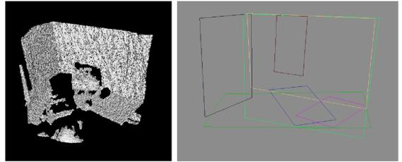
**Figure 4:** On the left, a 3D model reconstructed from raw depth data. SURROUNDWEB detects projectable “screens” to create the Room Skeleton, shown on the right. Web applications see only the Room Skeleton, never raw depth or video data.
