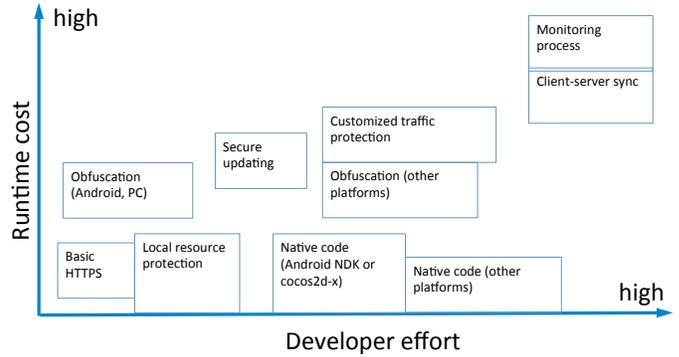
Figure 9: Protection cost comparison.
