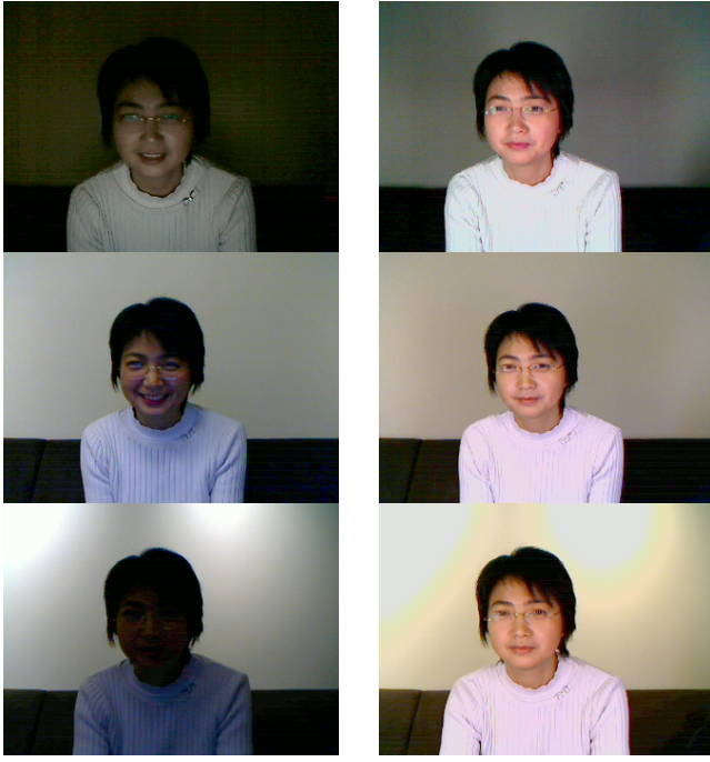
Fig. 9. Captured video frames in three different room lighting environment: dark room lighting for the top row, normal room lighting for the middle row, and back lighting for the bottom row. The left column are video frames captured without active lighting and the camera auto exposure is turned on. The right columns are video frames captured with the active lighting.
