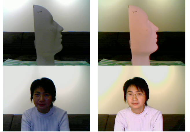
Fig. 14. Images for SNR evaluation where the room lighting environment is back-lighting. The images on the left column are obtained without active lighting but the camera auto exposure is turned on. The right column are images captured with active lighting.
