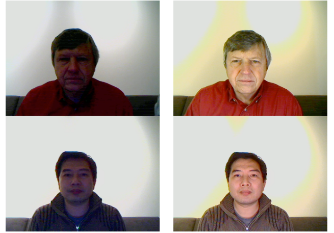
Fig. 11. Comparison of face-tracking based auto exposure vs. active lighting. The environment lighting is back-lighting where the wall is well lit while the face is dark. The images on the left column are obtained by using face-tracking based auto exposure control. The images on the right are captured with our active lighting system.
