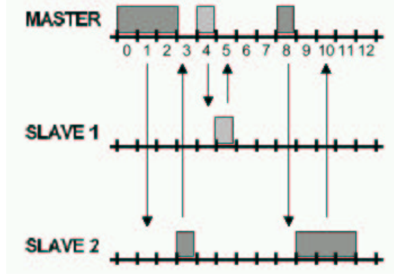
Figure 1.2: Frequency Hopping - Time Division Duplex Bluetooth MAC
