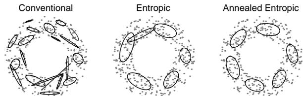
In the first case, over-fitting has resulted in a model of the accidental properties of the data (e.g., the clumpiness of the sample). In the second case, trimming has removed excess components and the resulting model looks much more like the essential structure of the data, but a large under-sampled region near the top still affects the model. In the third case, DA circumvents this local optimum and finds a model which generalizes even better.
