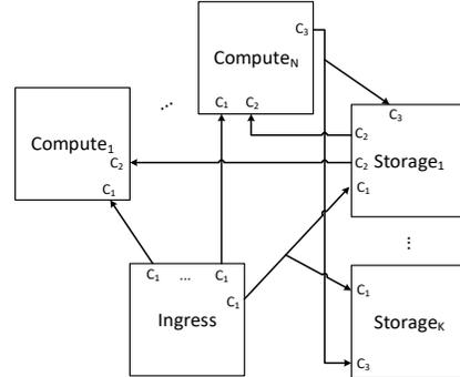
**Figure 11: Network Flow Diagram for Active-Active Periodic Checkpointing**
