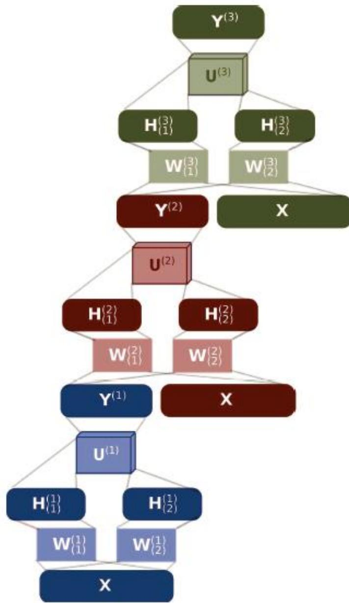
Fig. 1. An example T-DSN architecture with three stacking blocks, where each block consists of three layers, and
