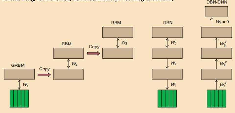
First train a stack of three models each of which has one hidden layer. Each model in the stack treats the hidden variables of the previous model as data.
