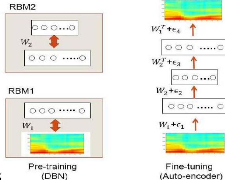
*Fig.1. Left: Illustration of pre-training of the DBN that consists of two RBMs used in this work. Right: Illustration of fine tuning that produces the final deep auto-encoder.*
