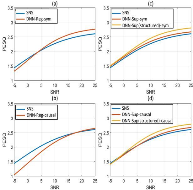
Figure 2: Output PESQ versus SNR for *unseen* noises. Note that the blue curve representing the performance of Statistical Noise Suppressor (SNS) is the same in all 4 figures and is provided for better comparison. *Left column*: Performance of DNN-based regression approach in causal (a) and symmetric (b) context modes. *Right column*: Performance of DNN-based suppression gain estimation approach in causal (c) and symmetric (d) context modes.
