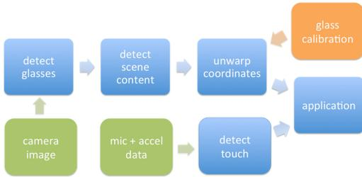
**Figure 2.** GlassHands processes image, microphone and accelerometer (green) to determine the glasses region, scene content and touch events. Calibration data (orange) is used to transform phone and hand coordinates from the camera’s image space to the display space of the phone.
