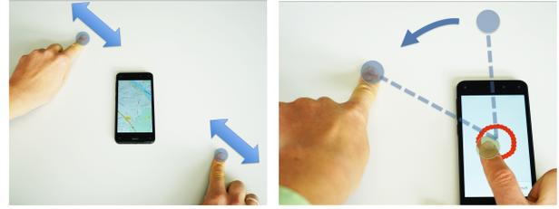
Figure 7. Left: Panning and zooming a map requires fewer repetitive gestures, compared to touch-screen only interaction and avoids screen occlusions. Right: The dominant hand draws on the touch display. The non-dominant hand rotates the virtual canvas around the screen center.
