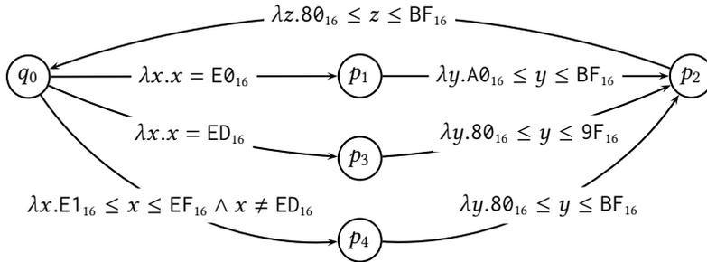
The same procedure is repeated for the fourth rule. After combining all the transitions together and minimizing [16] the resulting SFA we obtain the SFA in Figure 6 that accepts the range of *EncUTF8*.
