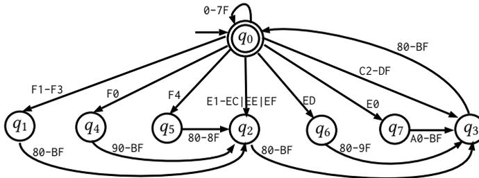
Fig. 6. Minimal SFA that recognizes valid UTF8 encoded strings.
