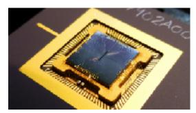
1152 superconducting qubits, D-Wave
