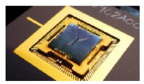
1152 superconducting qubits, D-Wave
