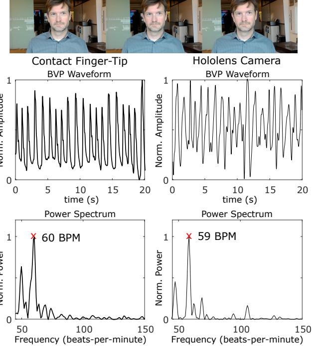
**Figure 5:** Examples of pulse waveforms from the finger-tip sensor and iPPG measurements. Top) The PPG waveforms. Bottom) The power spectra of the BVP signal and the detected HR. Thumbnail example frames from the Hololens video capture are shown above.
