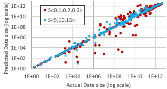
**Figure 11.** Accuracy of *PerfOrator* with profile runs at different sample rate combinations. The plot shows both the actual and predicted data-sizes for  $S\langle 0.1, 0.2, 0.3 \rangle$ ,  $S\langle 5, 10, 15 \rangle$ . The plot is in log-log scale
