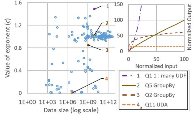
**Figure 4.** Input-output relationships: (on the left) values of  $c$  in  $output = b(input)^c$  for all stages of BigBench queries; (on the right) input-to-output behavior for four selected operators.
