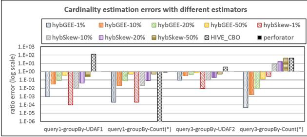
**Figure 2.** Comparison of cardinality estimates for UDA’s and deep pipelines. The figure shows the ratio error (predicted/actual) for different estimators. HybGEE- $x$  and HybSkew- $x$  are sampling based distinct value estimators ( $x$  is the sampling rate). HIVE\_CBO is the statistics based estimator used by Hive. PerfOrator is our system. Note : errors are plotted in log scale.
