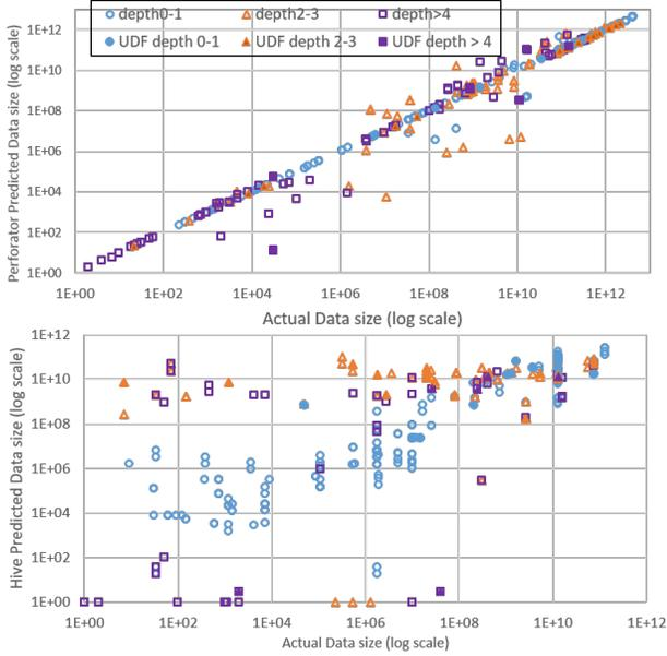
**Figure 10.** Accuracy of data-size estimation for *PerfOrator*  $S\langle 1, 2, 3 \rangle$  (above) and Hive (below). The plot is in log-log scale. Different colors are used to capture the depth of a stage within the query execution plan.
