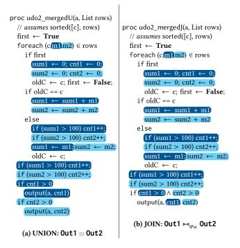
Figure 10: Merged UDOs for union (left) and join (right).
