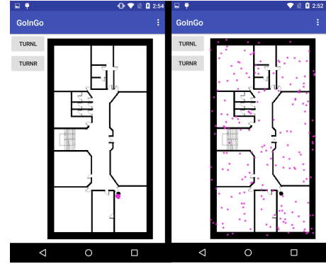
Fig. 3. An actual navigation in a room with 10-20 cm accuracy level using standard android smart-phone. Right:
