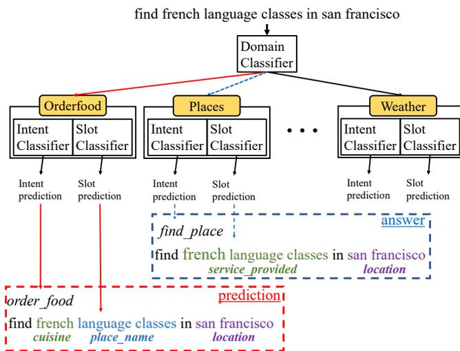
**Fig. 1.** Illustration of the pipelined procedure. If domain classifier predicted a wrong domain *Orderfood*, subsequent tasks – intent detection and slot tagging – would also make errors consequently.
