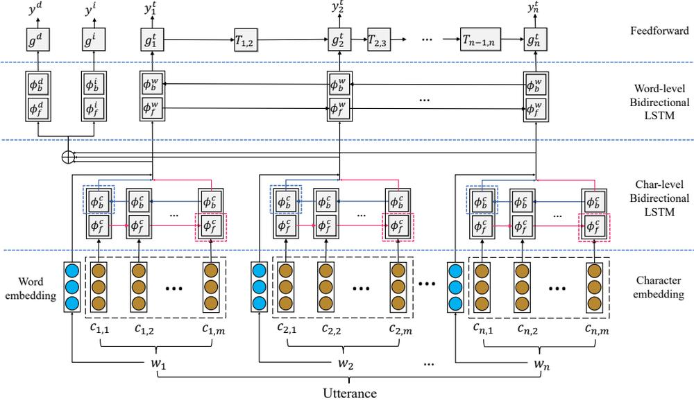
**Fig. 2.** The overall network architecture for joint modeling.
