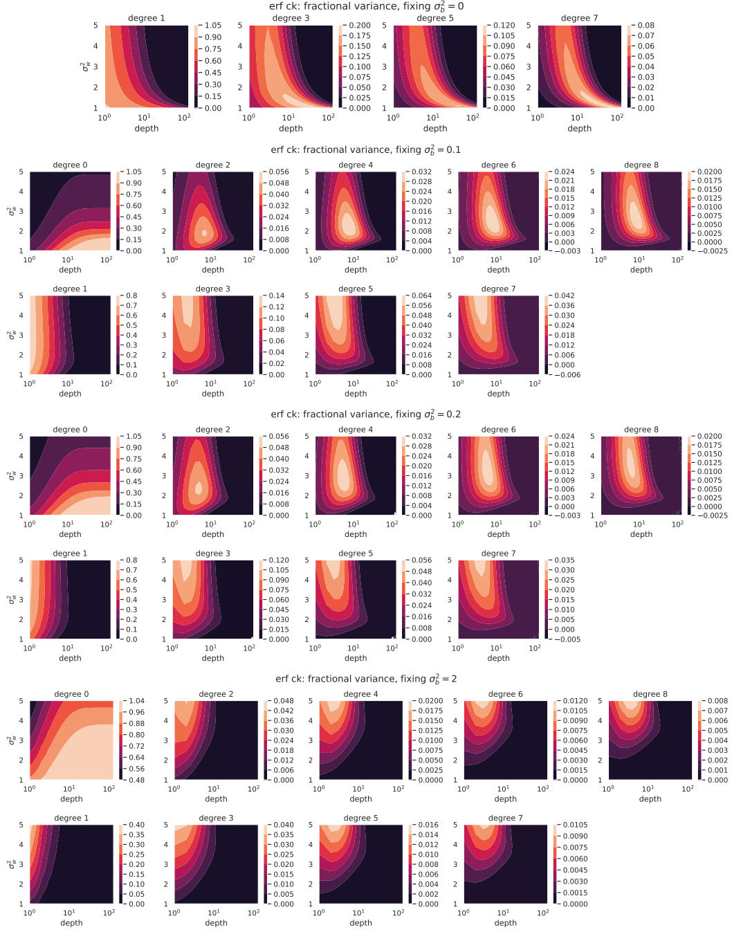
Figure 6: 2D contour plots of how fractional variance of each degree varies with \sigma_w^2 and depth, for different slices of \sigma_b^2 , for erf NTK. These plots essentially show slices of the NTK 3D contour plots in Fig. 8. For \sigma_b = 0 , \mu_k for all even degrees k are 0, so we omit the plots. Note the rapid change in the shape of the contours for odd degrees, going from \sigma_b^2 = 0 to \sigma_b^2 = 0.1 . This is reflected in Fig. 8 as well.
