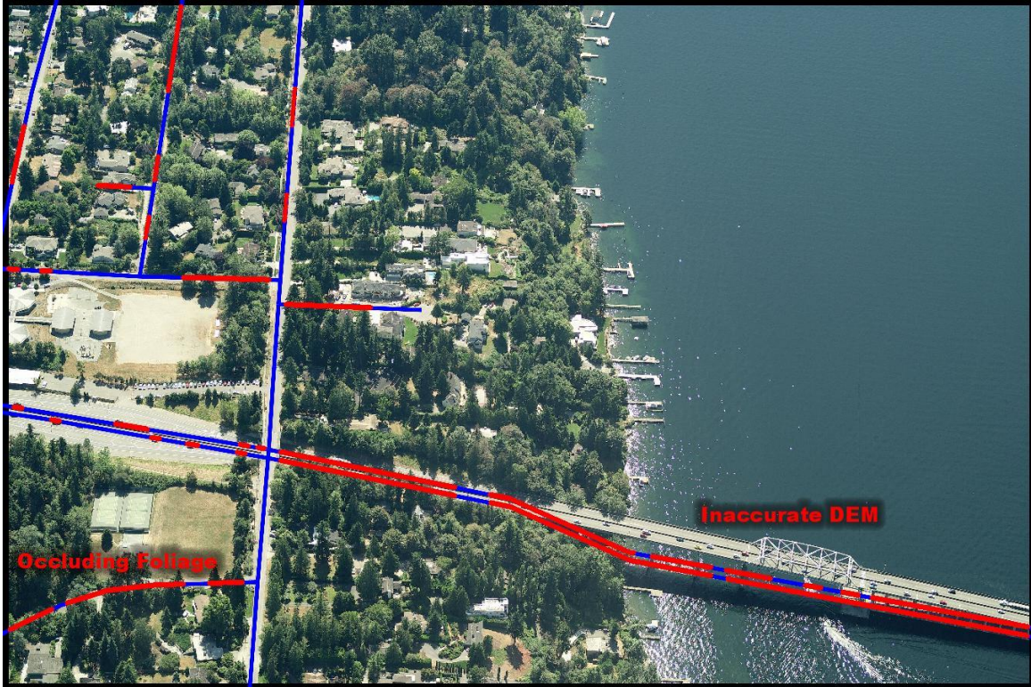
Figure 6. Road segments that are occluded by foliage or misaligned with their corresponding image areas due to inaccurate DEM are classified in red while consistent road segments are marked in blue.
