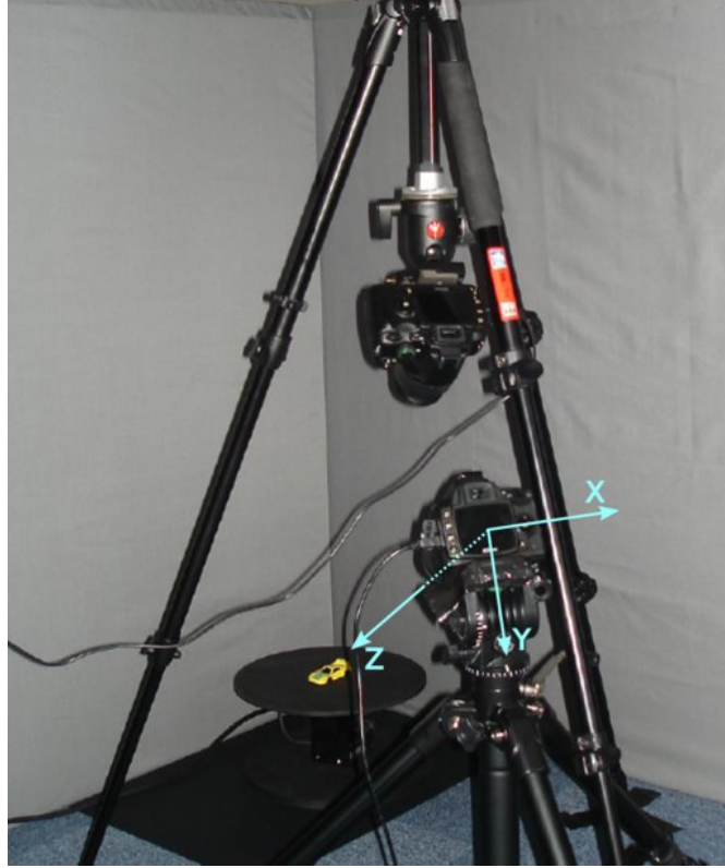
Figure 2: The rig used to capture the dataset. Note that the upper camera is inverted. All images from the upper camera are inverted, but no correction or de-rotation is necessary to handle this. All software provided assumes that the upper camera is inverted. The calibration process handles this correctly as the calibration images from upper camera are also inverted. If desired, the images may be de-rotated (by 180^\circ ) for display purposes.
