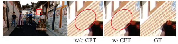
Figure 6. Example of without and with the cross-scale feature tokenization (CFT) on the REDS4 [29] dataset. CFT can transfer the clearer textures from larger scales to restore the detailed textures.
