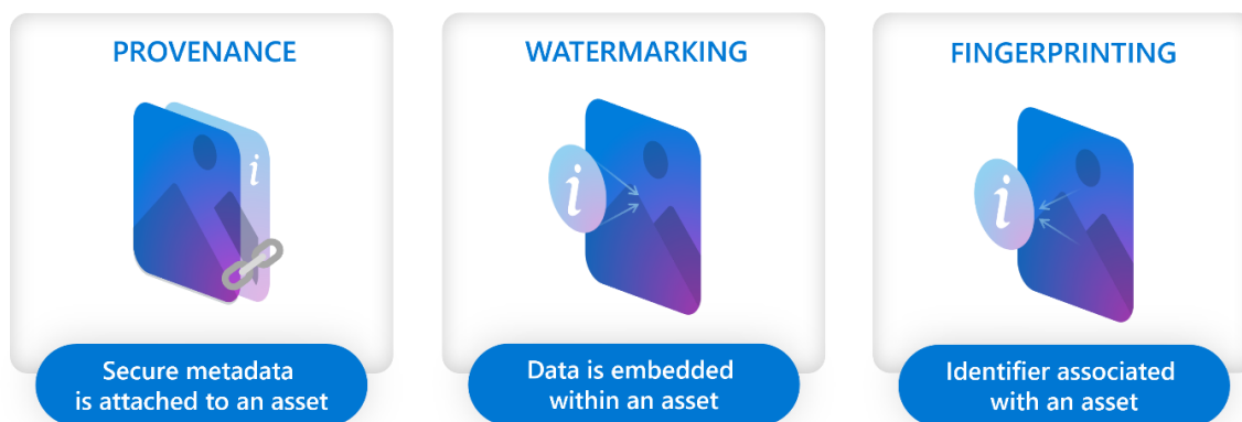
Figure 1: Simplification of provenance, watermarking, and fingerprinting media integrity methods.
