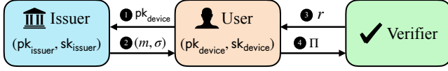
Figure 1. System model. During credential issuance (which happens infrequently), (1) the user’s client sends the public key of their secure element pk_{\text{device}} to the issuer; (2) the issuer produces and signs the credential m with its issuer secret key sk_{\text{issuer}} to produce signature \sigma and sends (m, \sigma) to the user’s client (the signed message includes the device public key). During zero-knowledge presentation (which happens many times) (1) the verifier sends a randomly sampled nonce r to the user; (2) the user’s secure element signs the nonce r with its device secret key sk_{\text{device}} and the user generates a zero-knowledge proof \Pi , where the proof establishes the knowledge of a signature on the nonce such that the signature verifies with the public key embedded in m (providing device binding, §3.1) and that the credential m is a valid credential (i.e., (m, \sigma) verifies using the public key of the issuer) and that attributes in m satisfy the verifier’s predicate.
