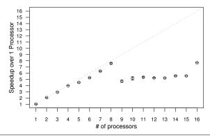
Figure 17. Multi-core performance for Huffman decoding
