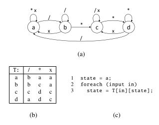
**Figure 1.** An FSM containing four states that accepts C-style comments in source code delineated by /\* and \*/. The input x represents all characters other than / and \*.
