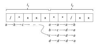
Figure 2. Enumerative computation for parallelizing FSMs.
